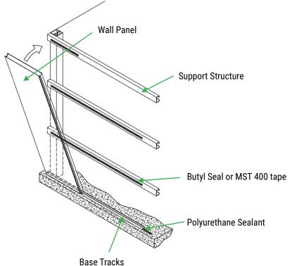
To begin with the installation of the panel, a 24-gauge base track should be installed.
