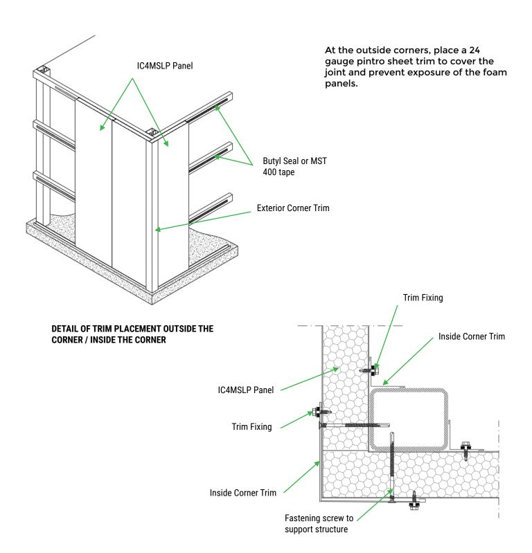
The panel is cut at each corner in order to have a better joint and tightness between the panels.
