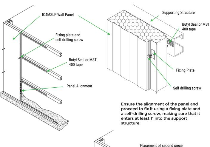
Once the first panel has been aligned and secured, the second piece of the panel is placed.
