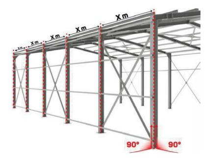
Before installation of the panels, it is necessary to check the alignment of the structure where the panel in use will be fixed, due to the possibility that the panel will adopt the irregularities that may exist in the structure.
