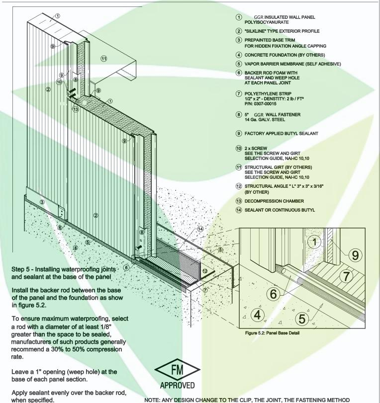
OR THE INSULATION PROPERTIES MUST BE COMMUNICATED TO FM FOR APPROVAL.
